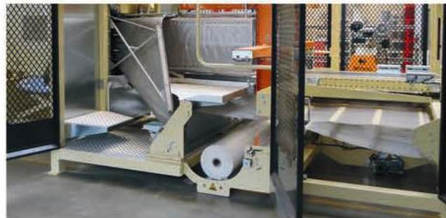
Our bales are shaped out of **flatfoil**. This offers advantages over so-called tubular foil or preformed bags; the foil may be thinner, less machining required, no bags in stock and much less material loss.
